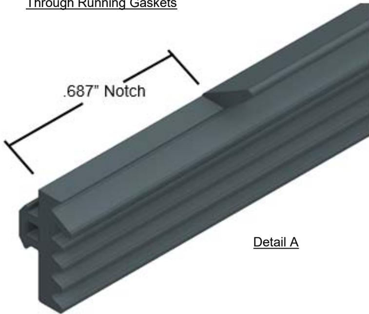
At through running pre-shim gaskets notch (see Detail A) both ends with the gasket outer finger portion fitting between the frame legs (Detail B). Through running pre-shim gaskets are to be installed first.
